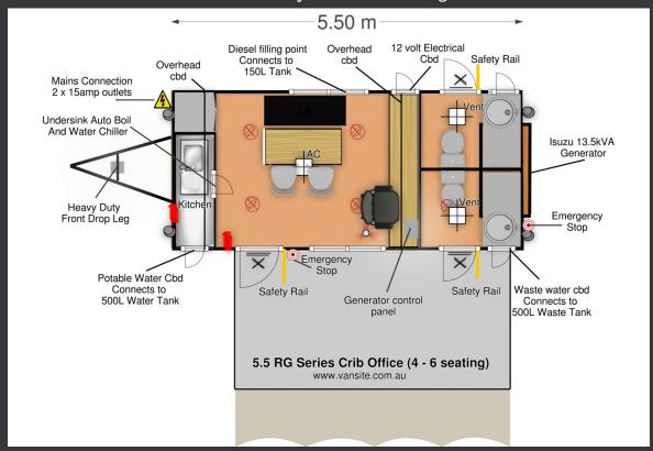
Our 5.5 RG series caters for larger crews up to 4-6 worker and is fitted with a separate toilets which can be use as Male / Female. This mobile office has a flexible layout which can cater for a large crib room or used as office space.
